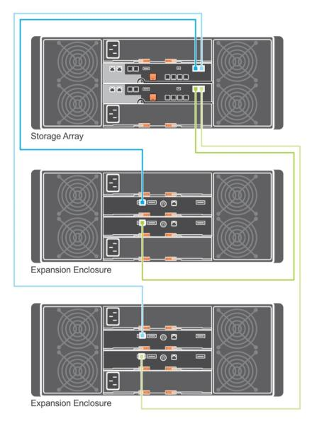
Figure 6. Dual expansion diagram
